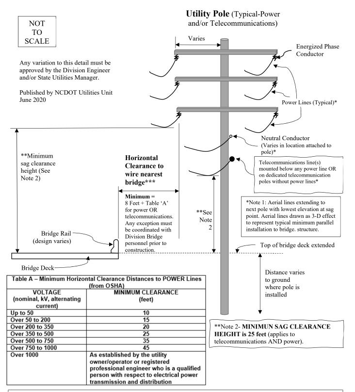
\*\*\*Note 3: HORIZONTAL CLEARANCE EXCEPTION. If vertical sag clearance height for power above bridge deck is  $\geq$  45 feet AND voltage is  $\leq$  350kV, then Minimum Horizontal Clearance may be reduced to 3 feet. Any telecommunications attachment to power pole allowed in this exception must have a minimum 25 feet sag clearance height above bridge deck.
